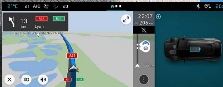
Energy flow : to visualise the electric flow from the battery
