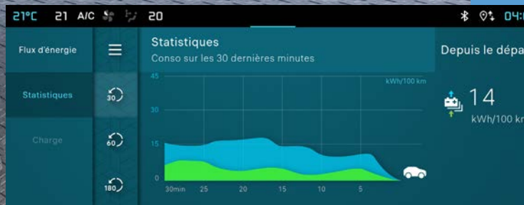
Statistics : showing electrical consumption to optimise driving
