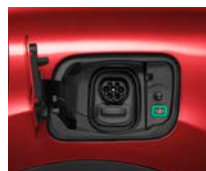
Charge Mode (Green diode flashing)
